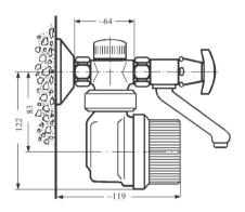
The mixer meter comes with a built-in closing device.
