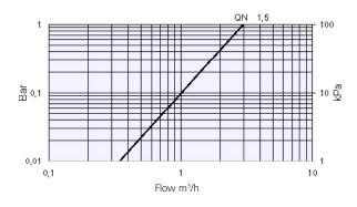
The head loss curve is valid for a meter without fittings
