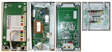
The conductors have to be fitted to the LSA-connector so the conductor is turned towards the cutting edge on the LSA-connector.
