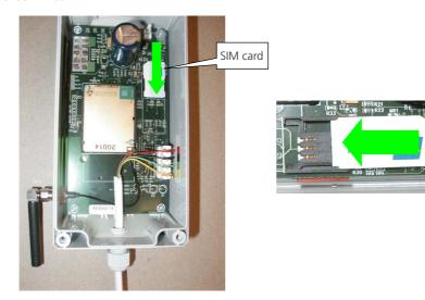
When the GPRS-box is on, the APN, log-in and pass-word must be installed so it corresponds with the operator of the SIM-card.
