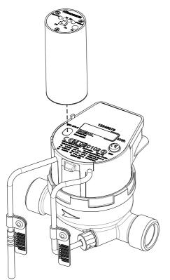
For correct configuration, the optical head must be placed on the optical interface. We recommend the Bluetooth optical head IZAR OH BT for configuration.
