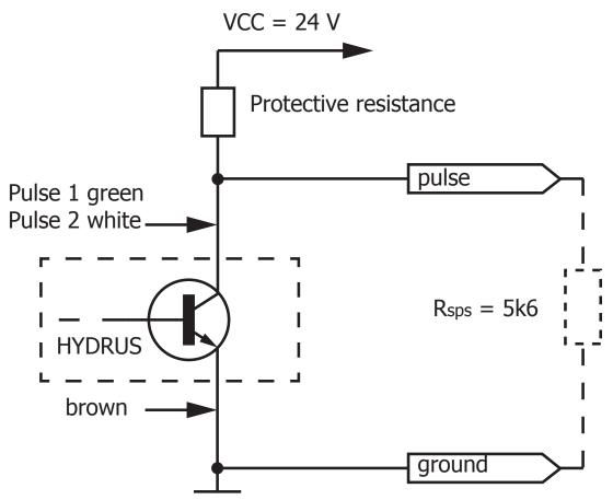
The pulse outputs are open-collector circuits.
